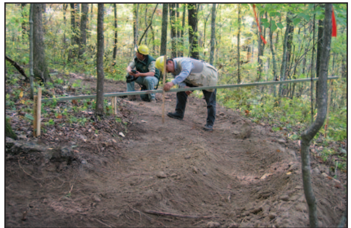
Figure 44—Rut depths of 1 to 4 inches were recorded.
